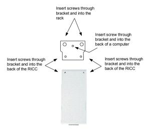
Figure 8 Rack mounting the RICC
